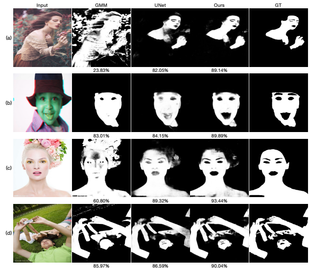
Figure 1. Skin detection results by our approach vs. solutions of a UNet and a tradition Gaussian Mixture Model (GMM). The intersection-over-union (IoU) rates demonstrate our approach has a better performance.
