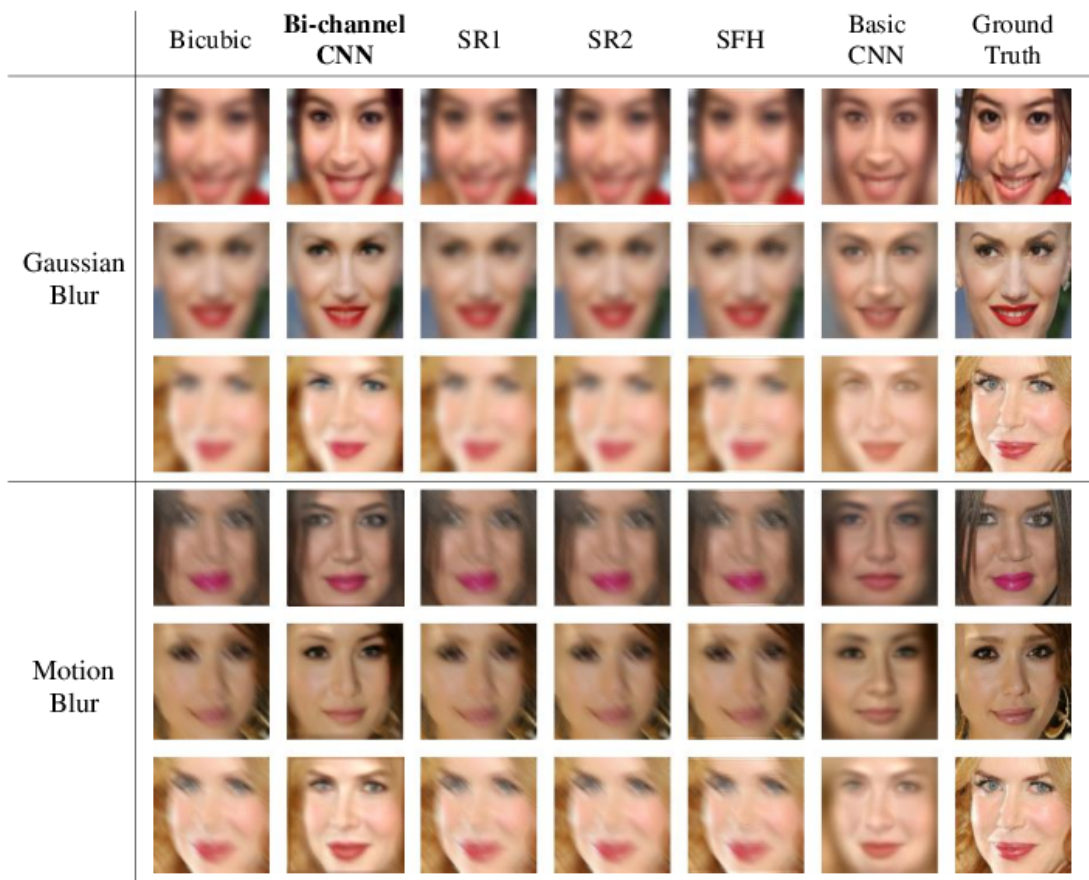
Figure 4: Qualitative comparison under different blurs. We compare the results from our system Bi-channel CNN with the results from generic super resolution method SC1 (Yang et al. 2008; 2010), SC2 (Kim and Kwon 2010), recent face hallucination method SFH (Yang, Liu, and Yang 2013), and Basic CNN. The results show our method outperforms the other methods in LR images with blurs. Best viewed in color.
