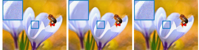
Figure 7. Image detail recovery. (a) Original noisy input image. (b) Filtered image by BM3D. (c) Defiltered image using our method. Note that the noise patterns between input and our recovered images are very close.
