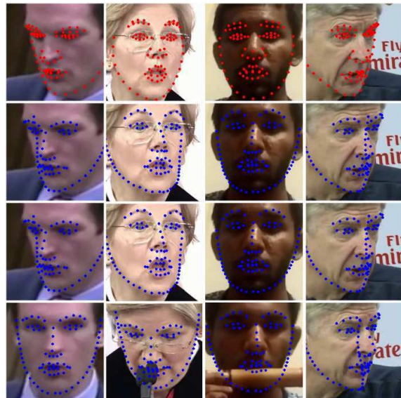
Figure 1. 3D face tracking results. The first row depicts the detection results of the first appearance of faces which is normalized with 81 2D landmark. Second row is the same image aligned with 84 3D landmark. Third row is the tracking results of the following frame, and the last row is randomly selected from the corresponding tracking sequences. Our tracking results perform well under various illumination, expression, posture, occlusion and blurriness.
