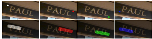
Figure 1. The images in top row and bottom row are the predicted corner points and position-sensitive maps in top-left, top-right, bottom-right, bottom-left order, respectively.
